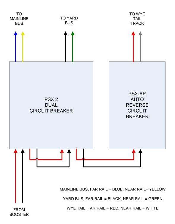
By April 8<sup>th</sup> I had fully wired the yard district. I used a bus of black and green of 12 gauge stranded wire for the yard district. The feeder wires are 22 gauge stranded wire. I used 12 gauge wire taps that I obtained through Mouser Electronics. The wire taps are made to accept a male quick disconnect terminal. One quick disconnect terminal is crimped onto each group of feeder wires.
