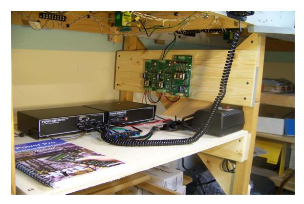
The layout has been divided into three power districts. The yard district is supplied by the one side of the PSX-2 breaker. The mainline and staging are supplied by the other side of the PSX-2 breaker. The PSX-AR auto reverse breaker supplies the tail of the wye.
